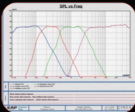
Response curves indicating the exemplary acoustic output of each filter network section with its associated transducers in a Salon2 loudspeaker
