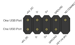
Figure : Dual USB2.0 pin-out(FP_USB2_1, FP_USB2_2)
