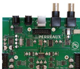
**éloquence DAC Module (Digital to Analogue Converter)**
