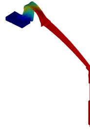
• Harmonic FEA model of the midrange driver assembly
