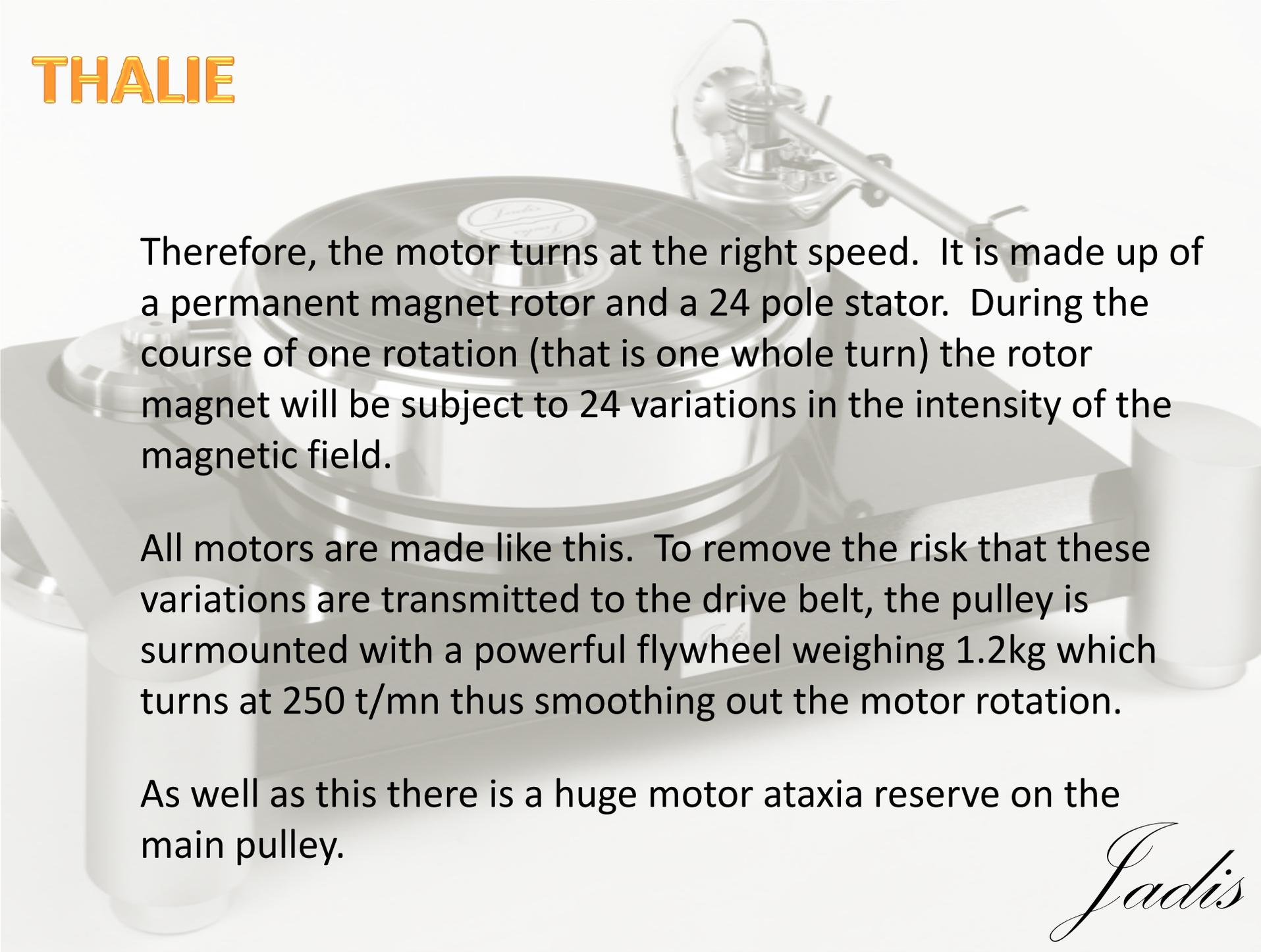
Therefore, the motor turns at the right speed. It is made up of a permanent magnet rotor and a 24 pole stator. During the course of one rotation (that is one whole turn) the rotor magnet will be subject to 24 variations in the intensity of the magnetic field.
