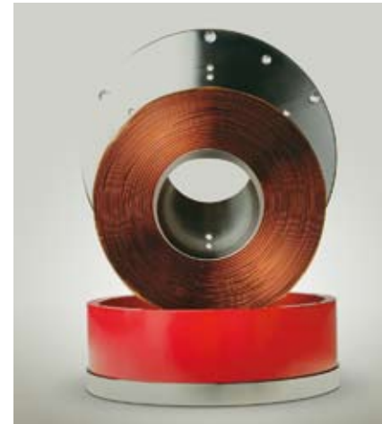
The EM Electro-Magnet is made of a 15.4lb (7kg) copper coil. The motor including the coil weighs 48.5lb (22kg). The 16" reaches a total weight of 52.9lb (24kg). "A monster" in the literal meaning of the word, where manufacturing costs cannot be compared to a standard magnet and are only conceivable on exceptional loudspeakers.
