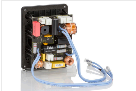
▲ BS 403, crossover and Van den Hul connection cables
