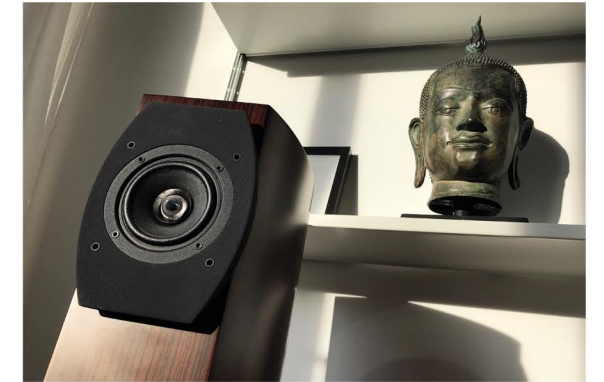
The 4" fullrange driver with whistler cone and active phaseplug implements the point source in our Comp 8 and Comp 9.
