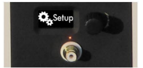
Our new operating concept with a rotary encoder and a graphic display allows an intuitive adjustment of all Loudspeaker paramters.
