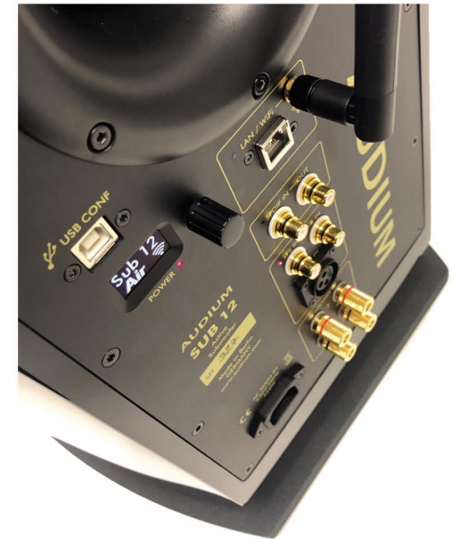
The user interface with rotary encoder and graphics display allows an intuitive setting of all Subwoofer parameters.
