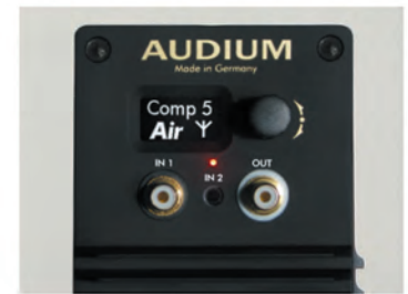
The Terminal of the Air Speaker: Display and Rotary Encoder, SPDIF Coax and TosLink (Phone Jack) Inputs and the SPDIF Coax Output
