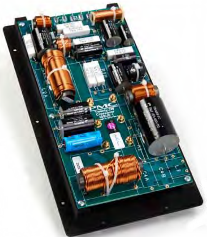
To seamlessly integrate the high, mid and bass drivers of the twenty.26 takes a highly complex and well-engineered crossover. It ensures the perfect supply of frequencies for each of the three drive units.
