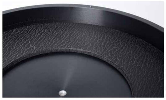
The heavy main platter of turned and anodised aluminium is generously dampened on the inside against vibrations and resonances: a layer of special foam soothes the surface, another layer of bitumen gives the damming sufficient mass and inertia.
