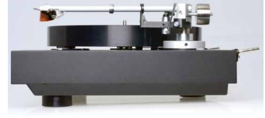
Barely visible from the side: owing to the subchassis, the platter bearing and arm base hover slightly above the surface of the PE chassis. Yet clearly recognisable from the side: the high-built 3 kg (6.6 lbs) aluminium platter and the upmarket TP92 tonearm from Thorens.
