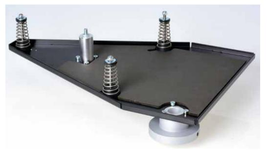
The heavy aluminium subchassis is lavishly dampened. The three conical springs are fitted with guide bolts against nutation and tensioned unevenly, as they are not centrically loaded. Above centre the platter bearing, the screw serves to fine-tune the weight uptake between ball and magnet.
