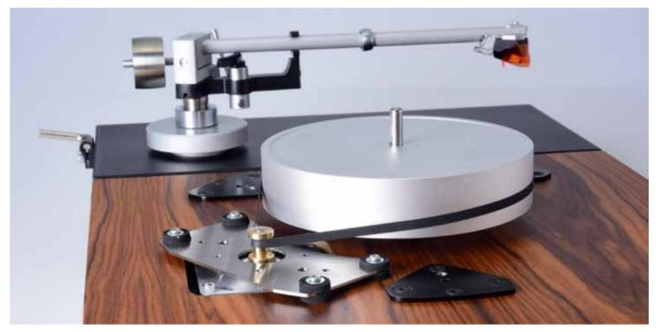
Damping all over: a wide belt provides the force transmission between motor (front left) and subplatter. Special feature: not only are the platter bearing and the arm base spring-suspended via the internal subchassis, but there are extra sorbothane dampers between outer chassis and motor plate and once again at the glued-in motor. The black plates are used to take up the six transport lock screws.
