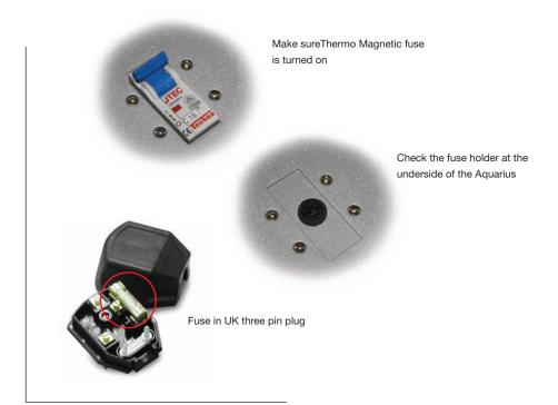
The front panel LEDs are not lit and the unit gives no power.
