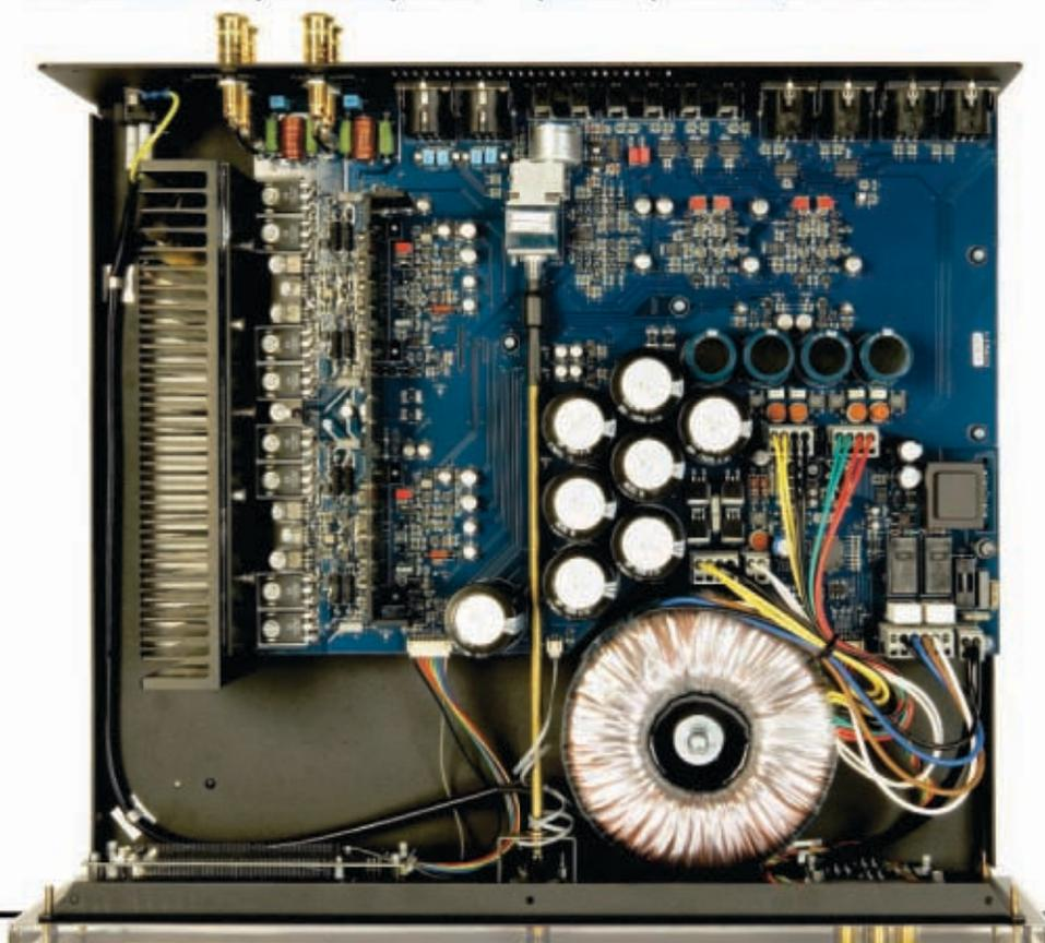
**RIGHT:** Internal changes in the MK II include a bigger mains transformer and reservoir capacitors, and, as seen on the left, the number of output devices has been doubled
