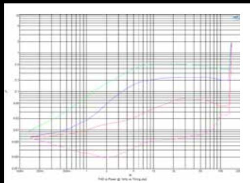
Small increases in dead-band time add significant levels of harmonic distortion. Shown are the relative levels of distortion from zero (theoretical, shown in purple) to 3 (red), 6 (blue) and 9ns (green) of dead-band time.
