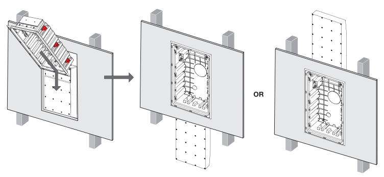
The reservoir box can be fitted within the wall either above or below the back box to enhance the speaker's low frequency performance. A clear distance within the wall should be reserved to accommodate the reservoir box.
