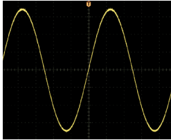
Photo (c) PS-1230 output waveform (distortion approx. 0.06%)
